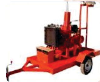
Trailer Mounted Pumps
